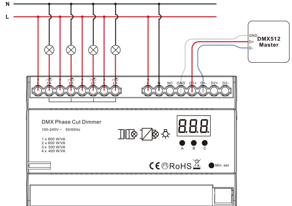
This phase dimmer adopts trailing edge dimming (reverse phase control), the dimming range is 1%~100%, please make sure the connected loads support reverse phase control. Please refer to the user manual of the load or consult the supplier of the load.
